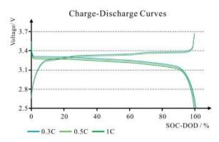
Note: Due to the ultra-high rate battery, there is almost no difference between 0.3C and 1C capacity.
